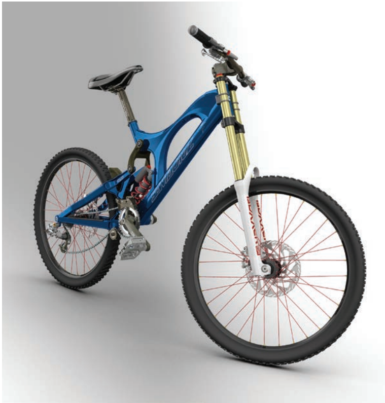
1.10 The V10 is a generation of downhill racing bikes first sold in 2002 and continually improved based on race team results and rider feedback. The 3D model of the new design is shown here. (Courtesy of Santa Cruz Bicycles.)
